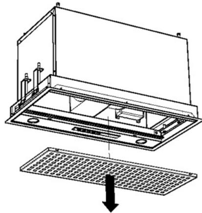
Protect the cooking plate. You can take the grease filter out of the hood by pulling the handle that has been placed on the filter. The filter will come down.
